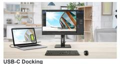
Simplify the connections with one cable only. The USB-C connection provides DisplayPort Alternate Mode for transferring high-resolution video signals from a notebook to the monitor while simultaneously charging the notebook's battery from the monitor with USB power delivery.
