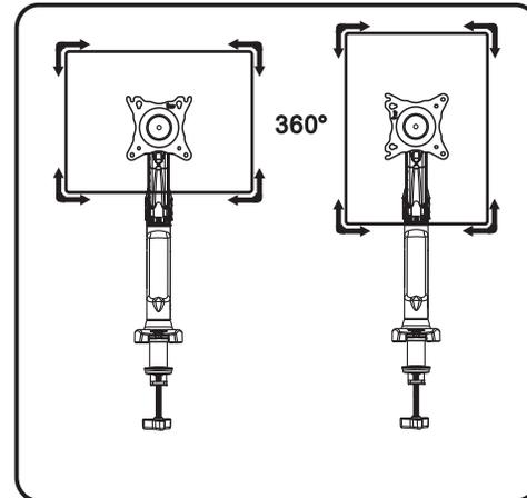
AFTER INSTALLATION, ADJUST GAS-SPRING POWER
