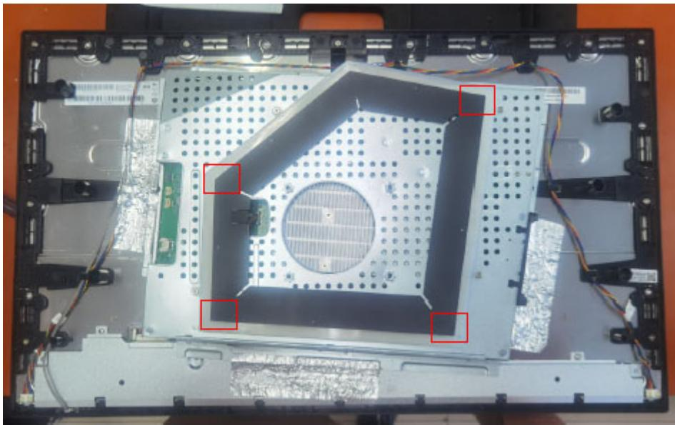
4. Remove the screws, Disconnect the connection.
