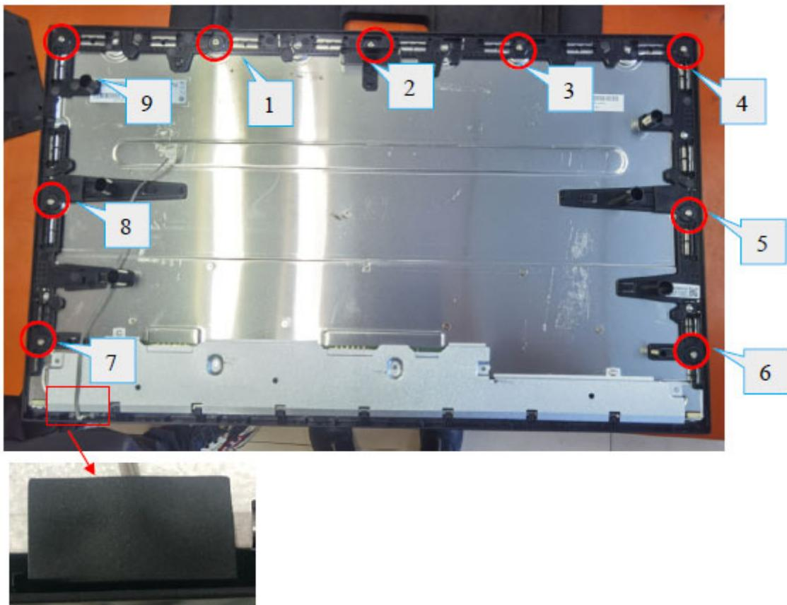
7. Remove the screws to remove the boards. Disconnect the connection.
