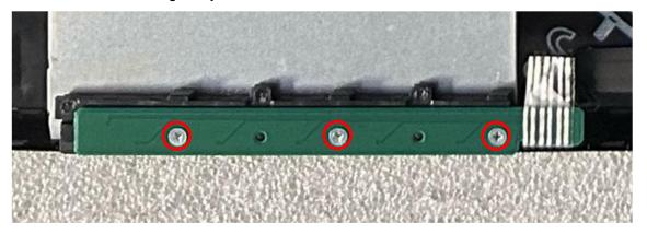
12. Remove screws then the middle frame you can get the panel.
