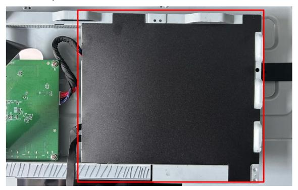
10. Remove screws to get main board and power board.
