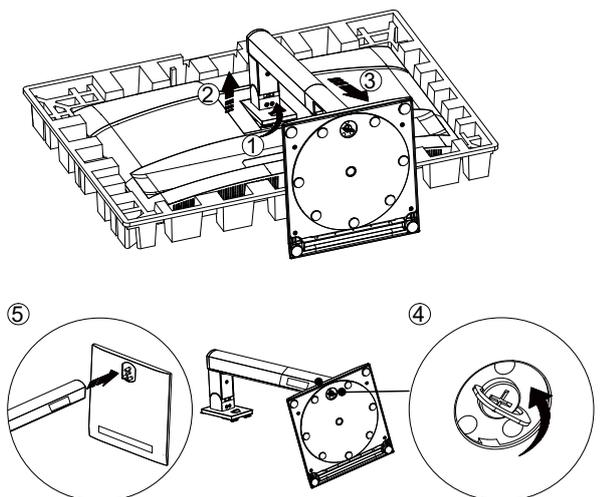
Specification for base screw: M6\*17 mm (effective thread 5.5 mm)
