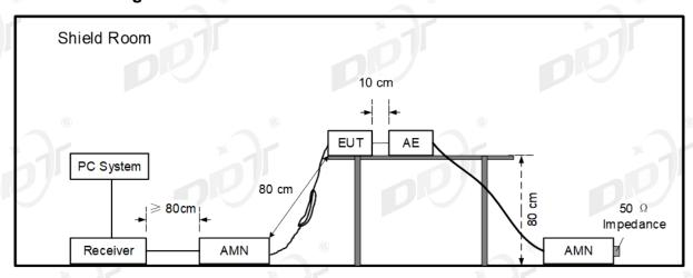
The EUT was placed on a non-metallic table, 80cm above the ground plane.
