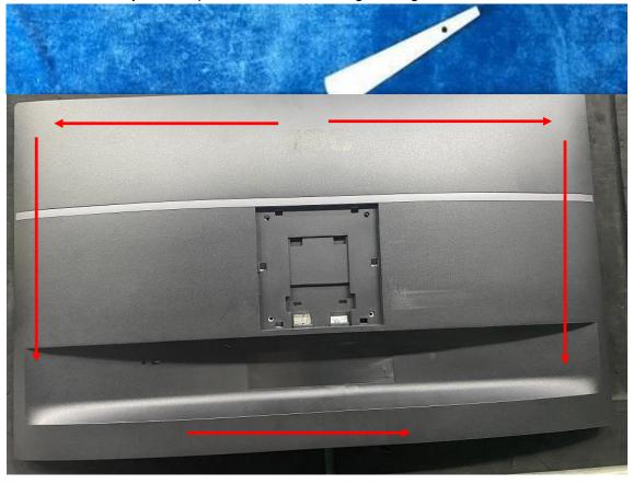
4. Take off the tape and disconnect connectors, then you can remove the rear cover.
