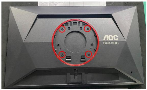
4. Use disassembly tool to open all the latches along the edge of rear cover.
