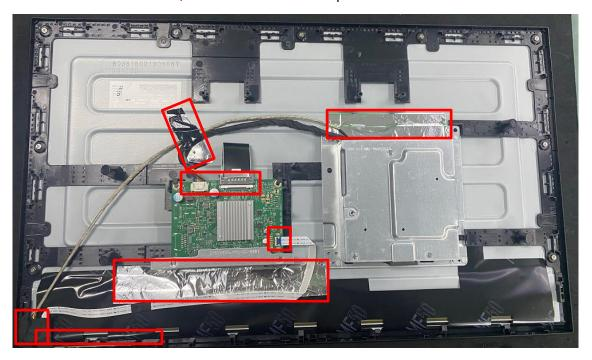
6. Remove mainframe and screws.
