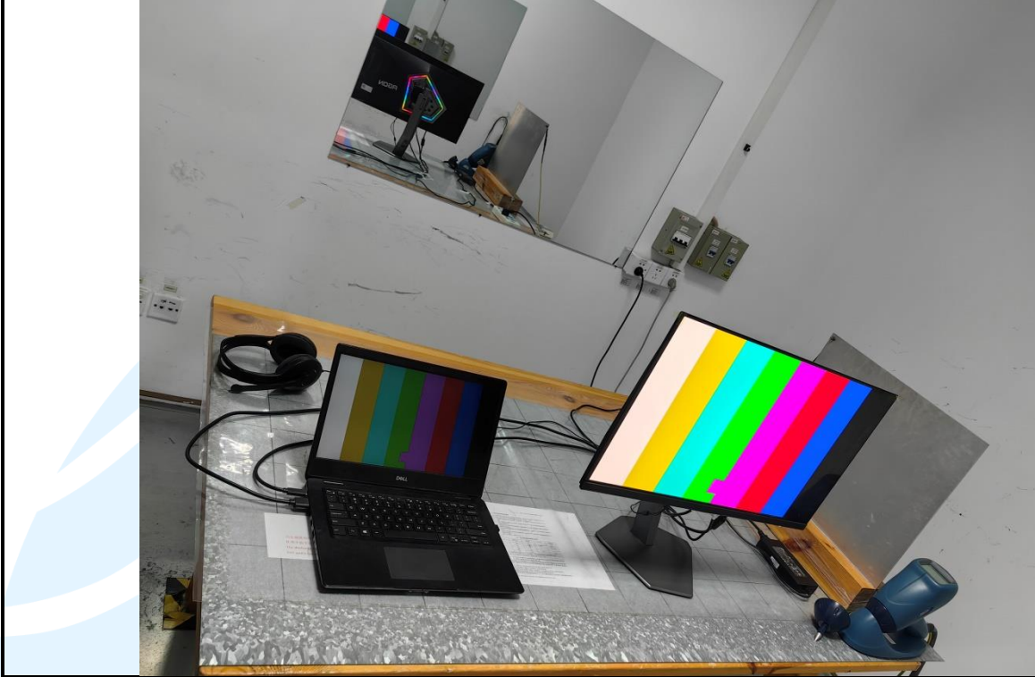
Electrostatic Discharge Test Setup
