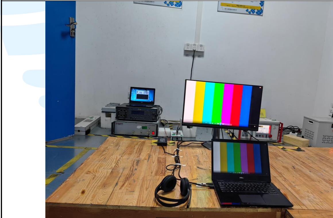
Radio frequency, common mode (AC Port) Test Setup
