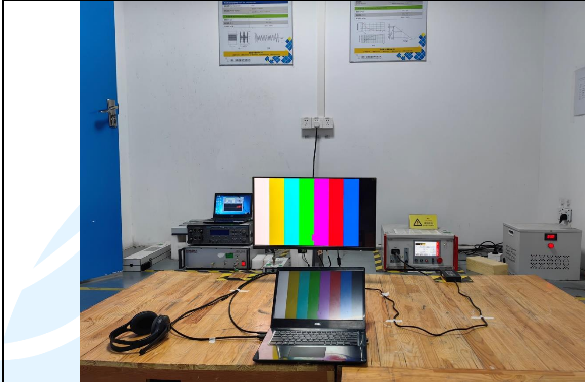
Fast Transients, Common mode / Surge Test Setup (AC Port) Test Setup
