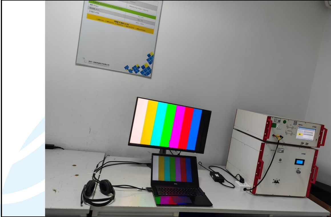
Voltage dips and interruptions Test Setup
