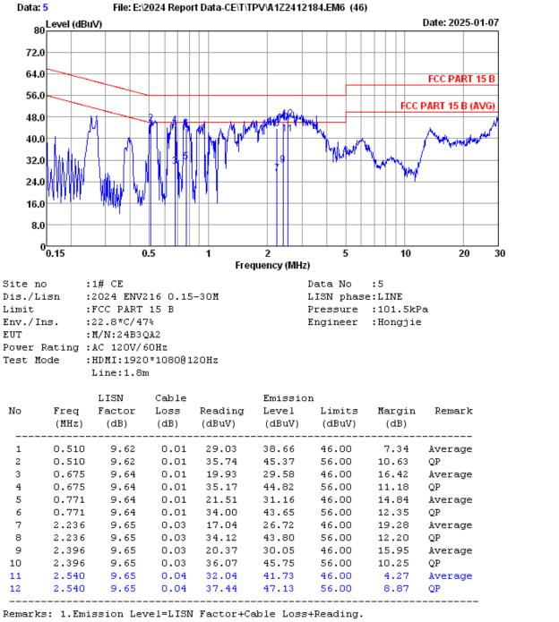
2. If the average limit is met when using a quasi-peak detector. the EUT shall be deemed to meet both limits and measurement with average detector is unnecessary.
