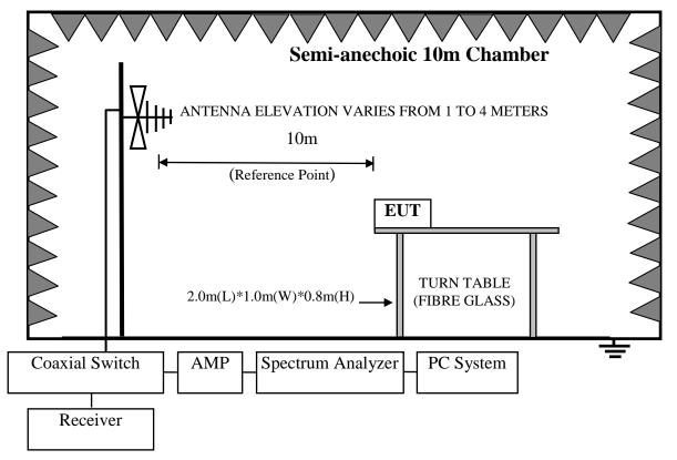
4.2.2. For frequency range above 1GHz (In 10m Anechoic Chamber)
