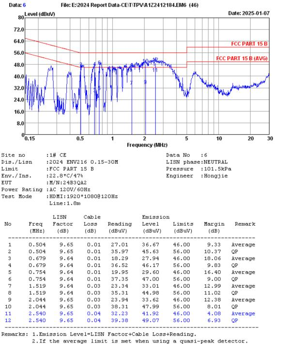
the EUT shall be deemed to meet both limits and measurement with average detector is unnecessary.
