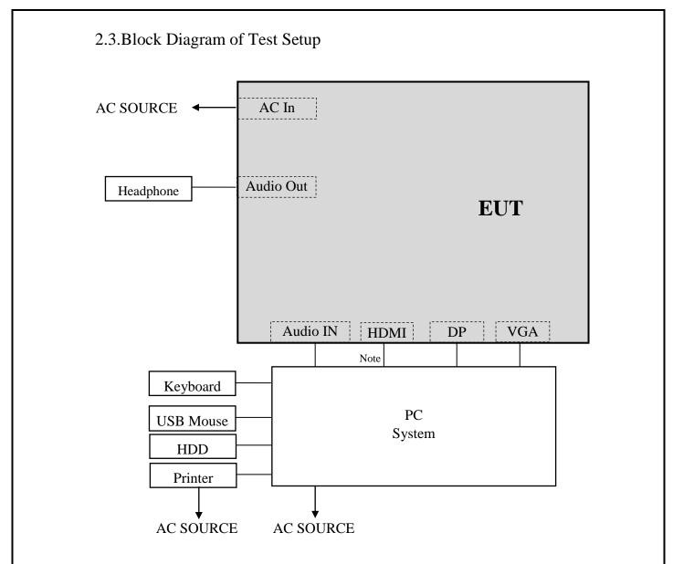
Note 1: PC Mode, DVD Mode can not link the HDMI port at the same time. (EUT: LCD Monitor)
