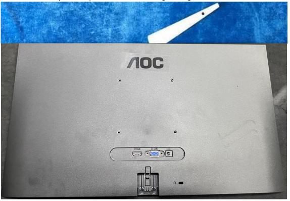
4. Disconnect the connector then remove the rear cover.
