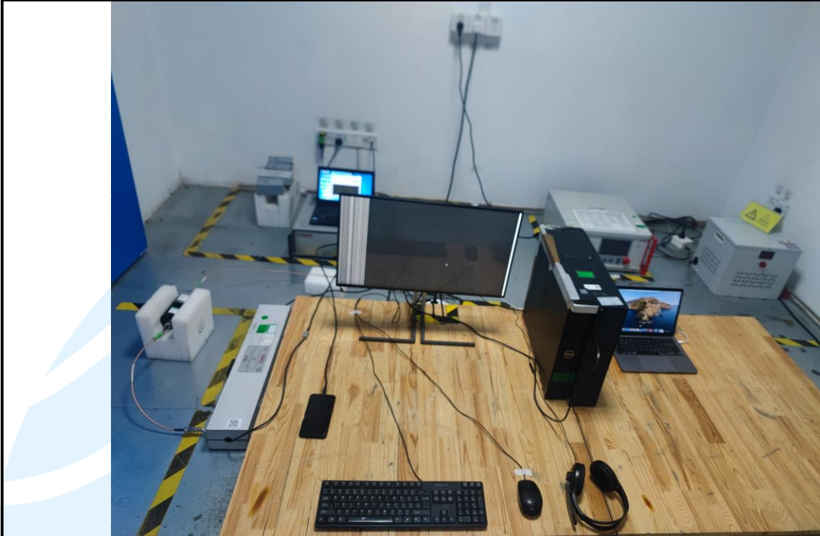
Radio frequency, common mode (Wired network ports) Test Setup
