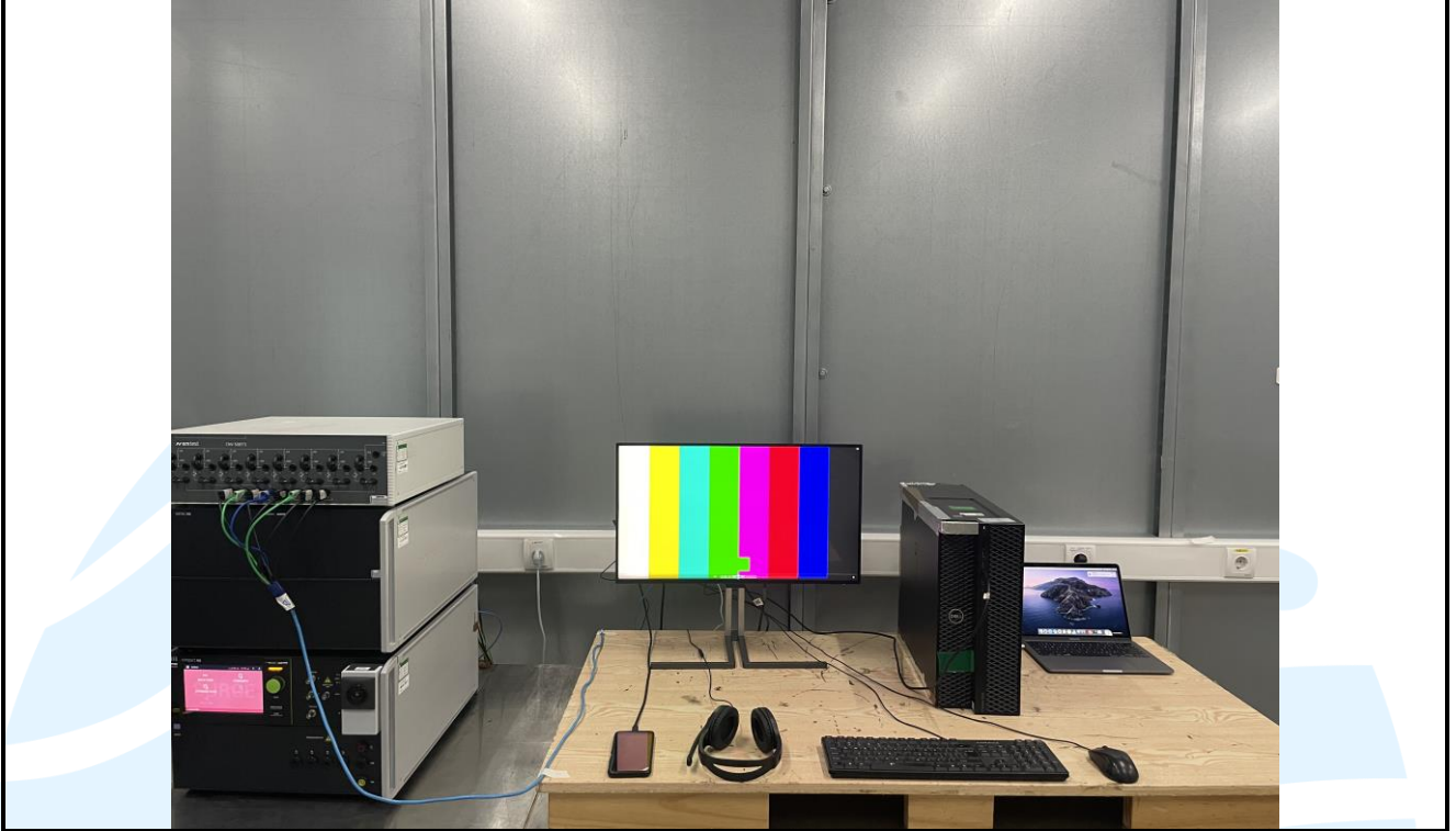
Surge Test Setup (Wired network ports) Test Setup
