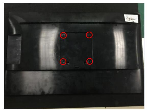
4. Use disassembly tool to open all the latches along the edge of rear cover.
