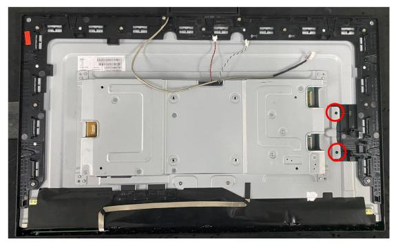
8. Throw the main frame from one side, take off the tape and disconnect the connectors. Then remove the main frame.
