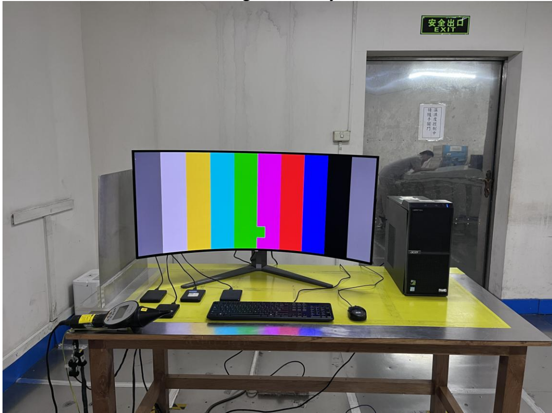
15.4. Photos of Electrostatic Discharge Immunity Test
