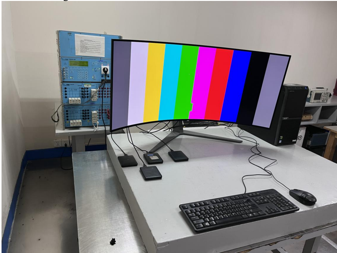
15.7. Photo of Surge Test
