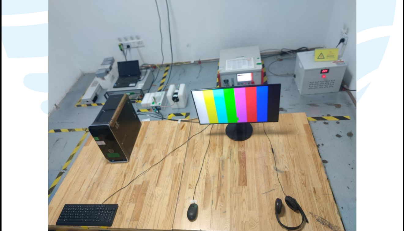
Fast Transients, Common mode / Surge Test Setup (AC Port) Test Setup
