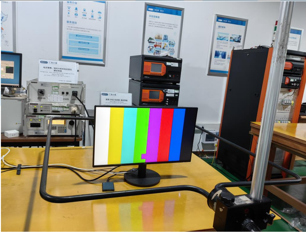
Power frequency magnetic field Test Setup
