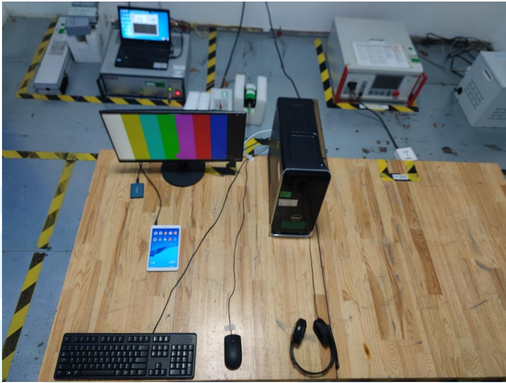
Radio frequency, common mode (AC Port) Test Setup
