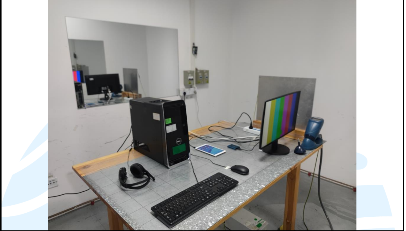
Electrostatic Discharge Test Setup
