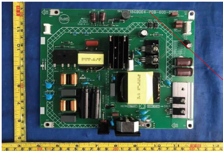
Photo 6 - Power Board (715GB004)
