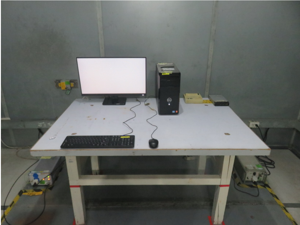
AC Power Line Conducted Emissions
