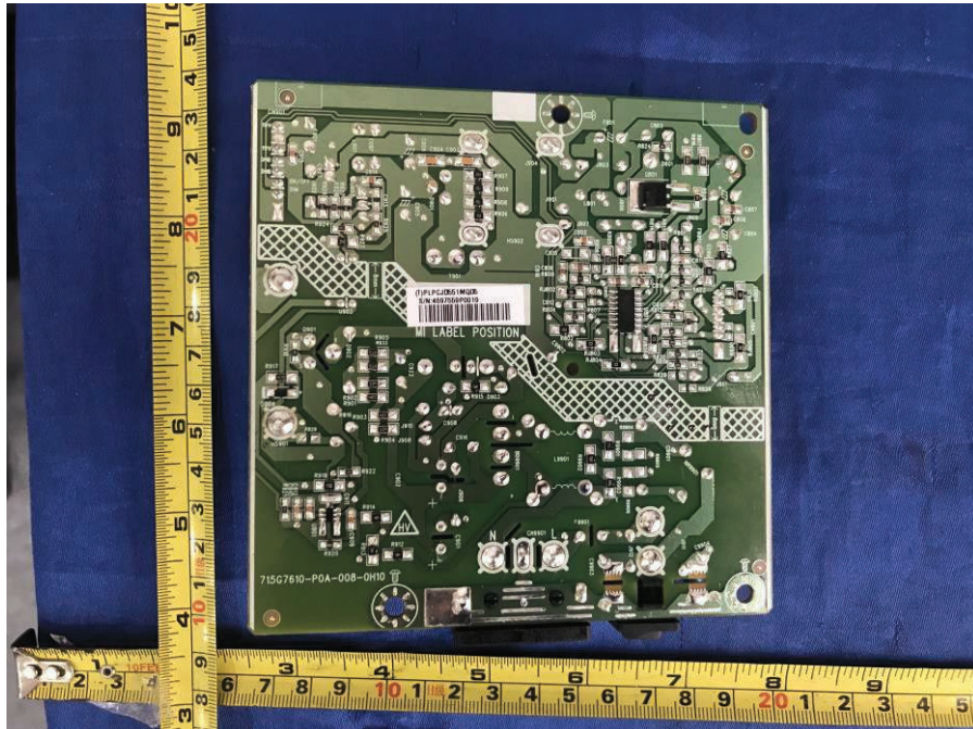
Figure 15. Power board 715G7610
