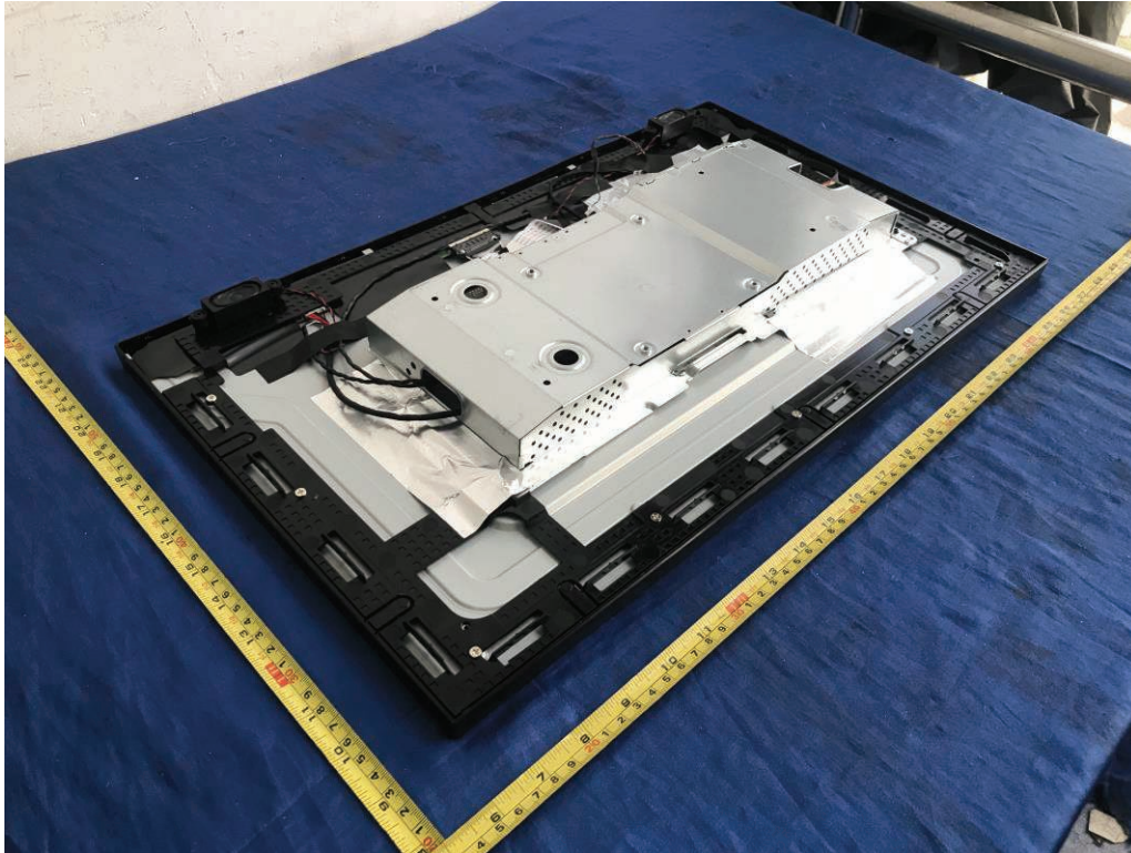
Figure 7. Internal view of 23 inch models
