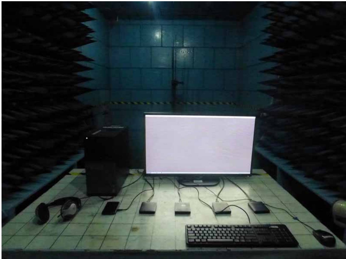
15.5. Photo of RF Strength Susceptibility Test
