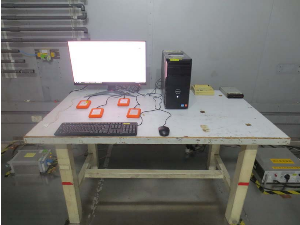
AC Power Line Conducted Emissions
