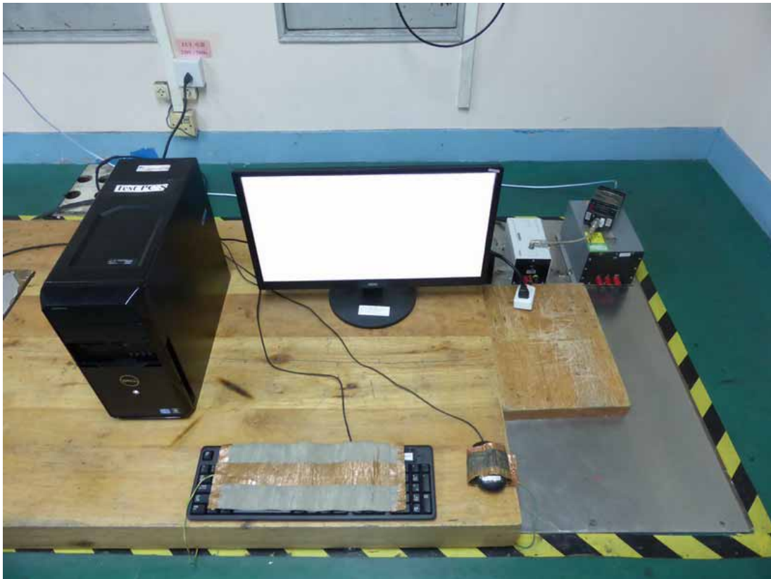
15.8. Photo of Injected Currents Susceptibility Test
