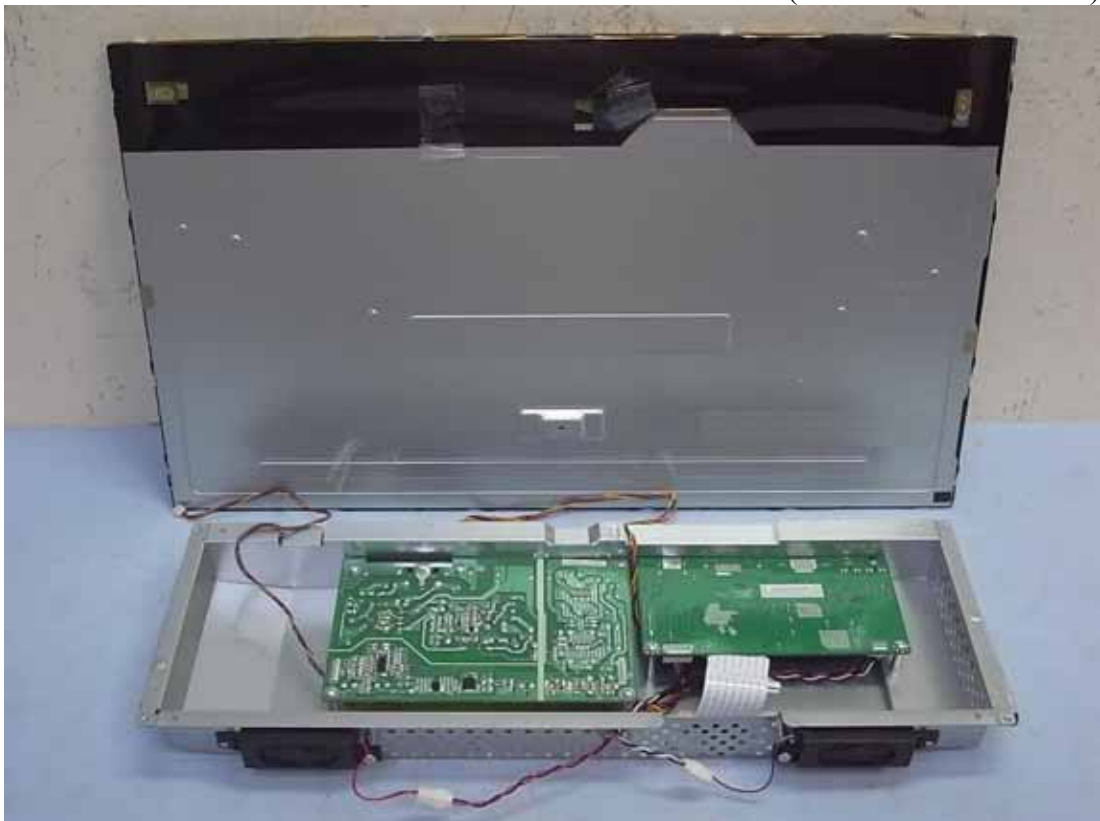
Figure 8 Internal View (Removed Metal Cover)
