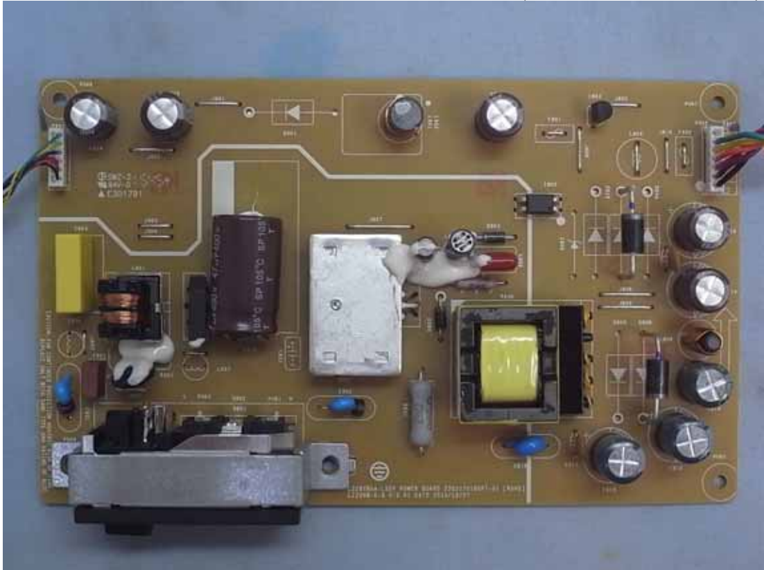
Figure 11 Internal View (Power Board, Front View)
