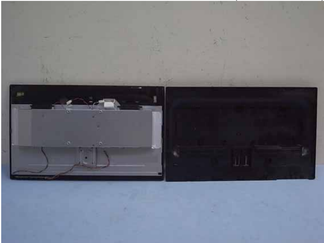
Figure 21 Internal View (Removed Back Cover)
