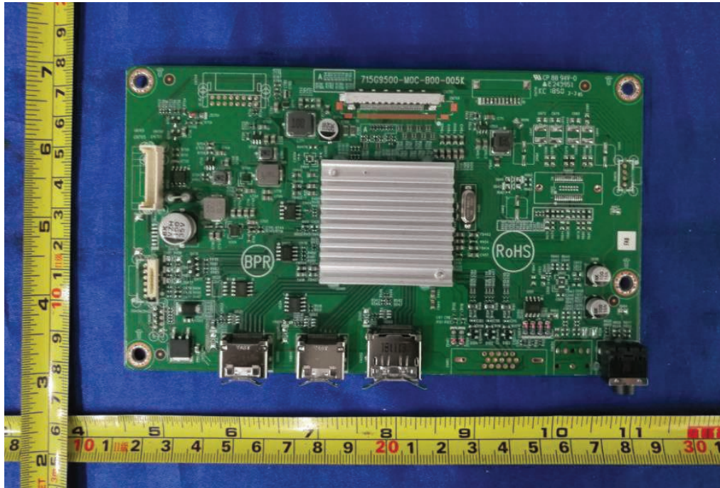
Figure 11. Main board 715G9500 used for models 27G1, **27G1*****
