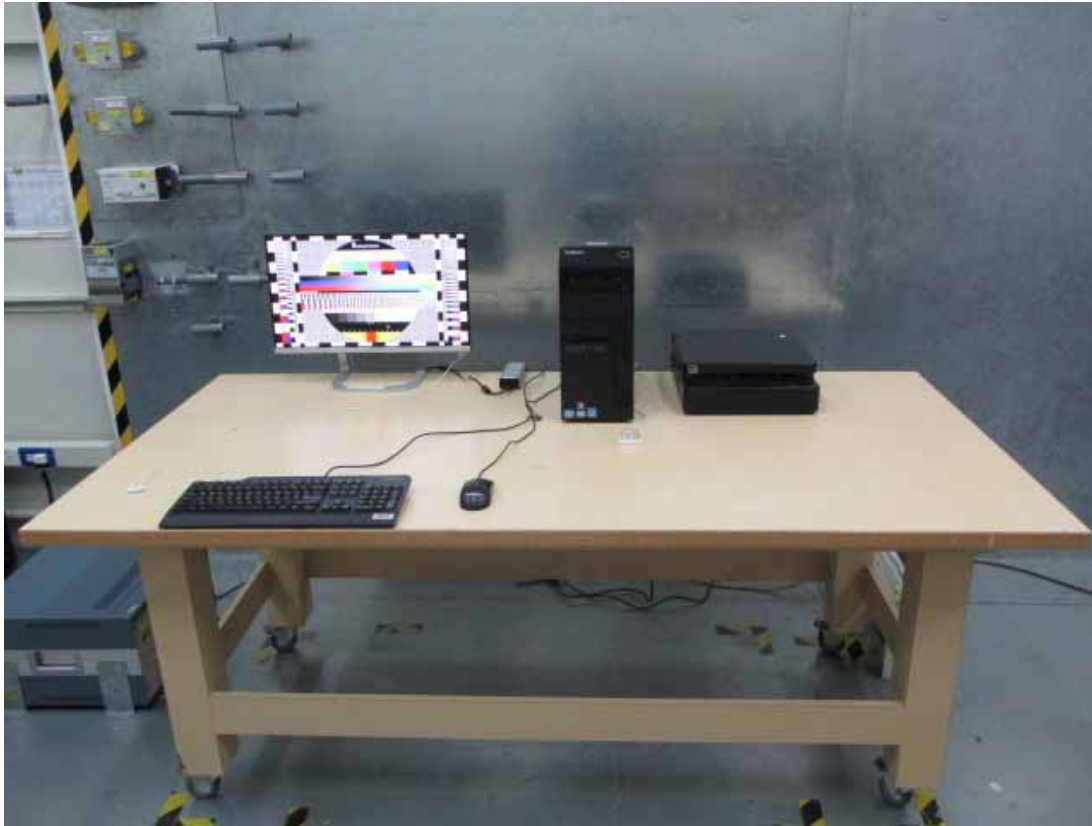
Front View of Conducted Measurement
