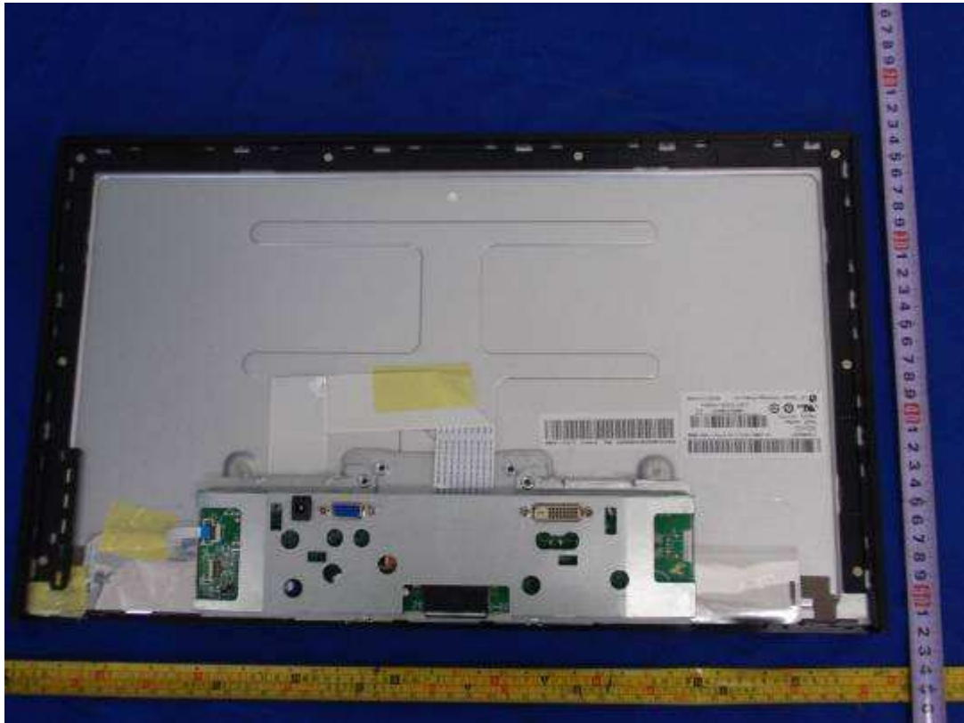
Figure 9 Internal view of 20" model with main board 715G5233
