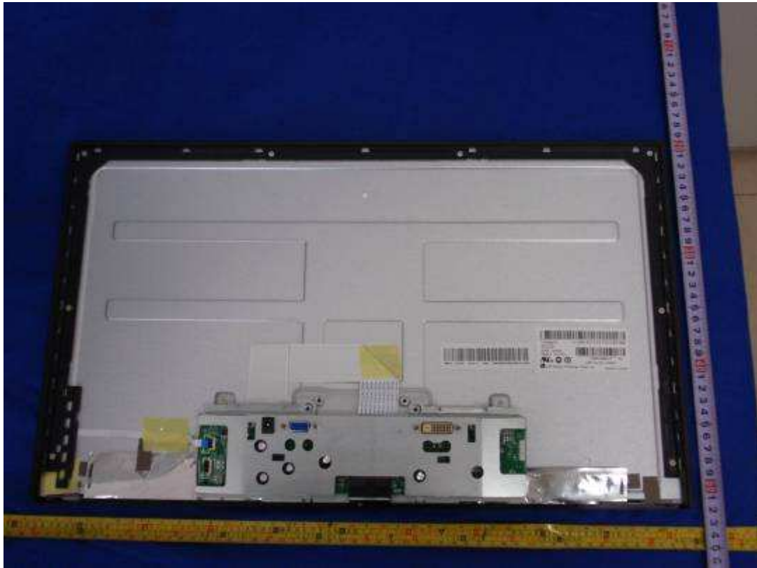
Figure 11 Internal view of 23" model with main board 715G5633
