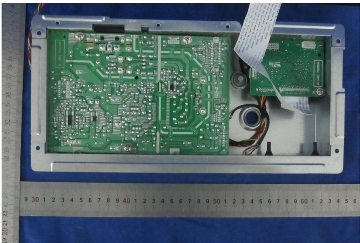
Fig.4 _ Internal view with power board without mylar sheet (type: 715G4497)
