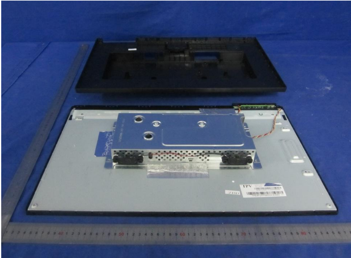
Fig.1_ Construction with internal speaker
