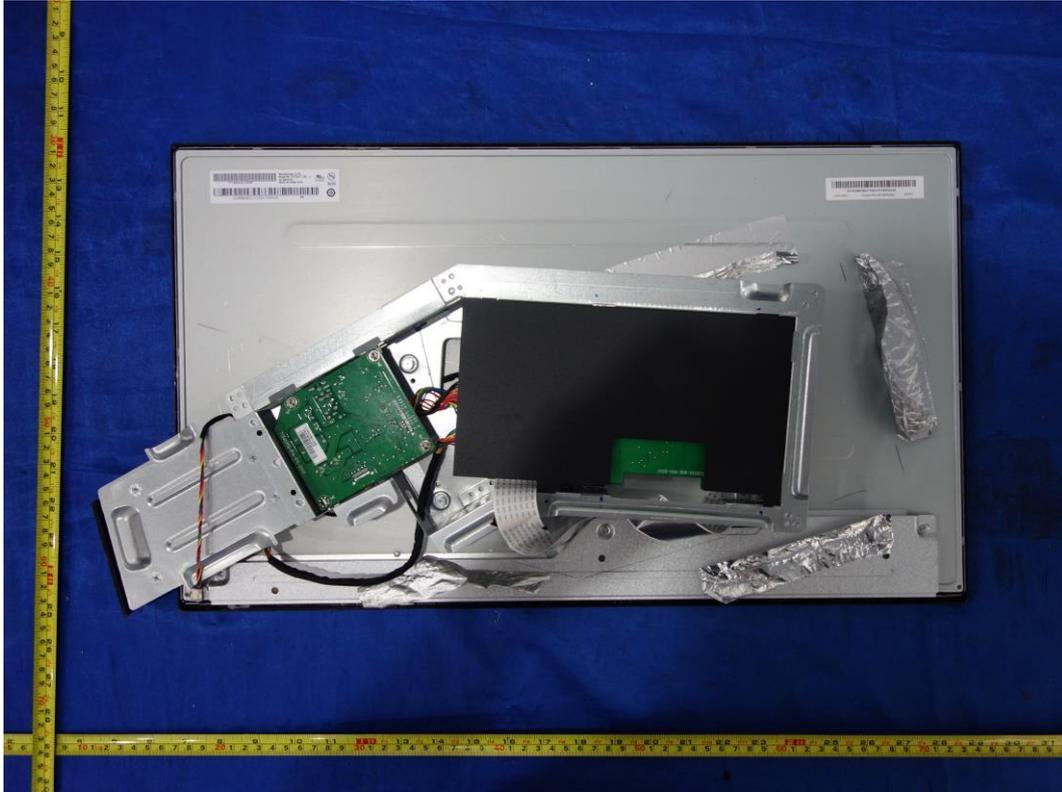
The internal view with mainboard type C
