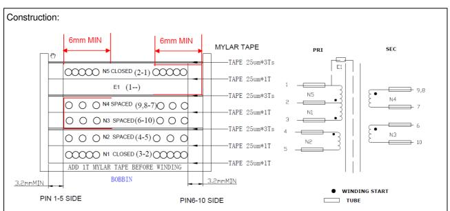
Concentric windings on phenolic bobbin. Three layers insulation tape are provided around outer winding and outer winding is primary. There layers of insulation tape are provided between the primary windings and secondary windings. At least 3.2mm margin tape is provided for primary windings and at least 3.2mm for secondary windings. Two layer of insulation type is provided around the core. All winding leads are covered by tube.
