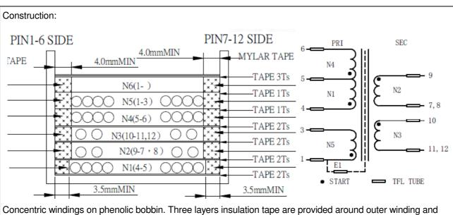
Concentric windings on phenolic bobbin. Three layers insulation tape are provided around outer winding and outer winding is primary. Two layers of insulation tape are provided between the primary windings and secondary windings. At least 3.5mm margin tape is provided for primary windings and at least 4.0mm for secondary windings. Two layer of insulation type is provided around the core. All winding leads are covered by tube.
