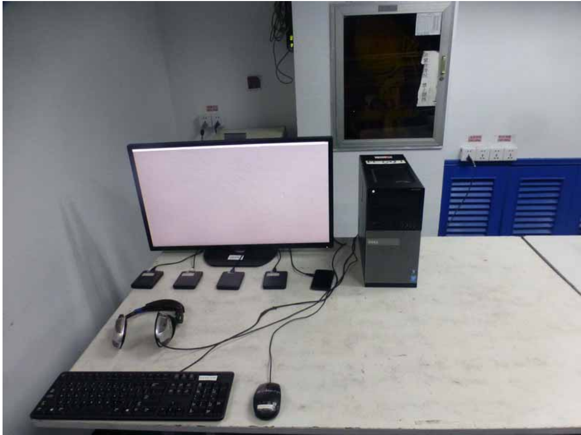
15.10. Photo of Voltage Dips and interruptions test
