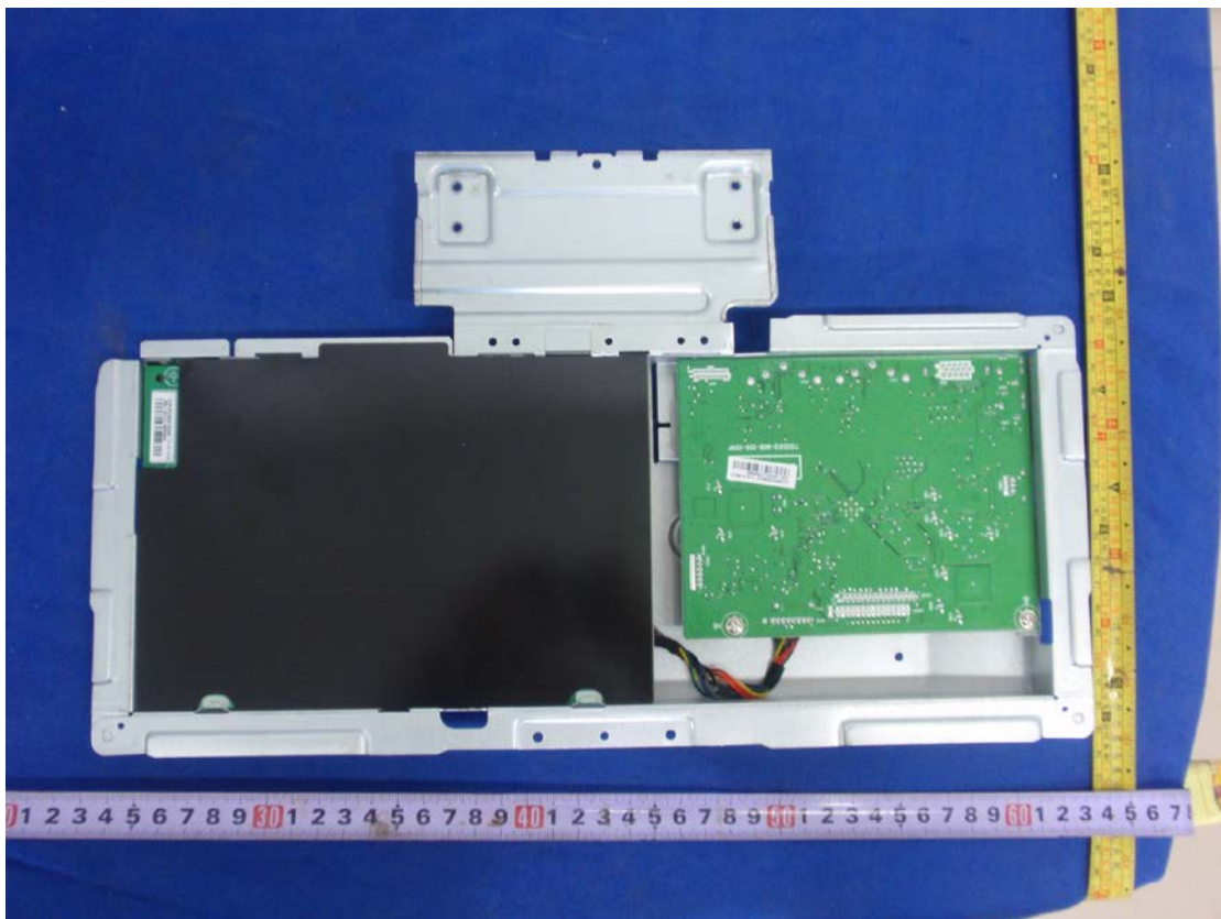
Figure 24. Internal view with main board 715G5812
