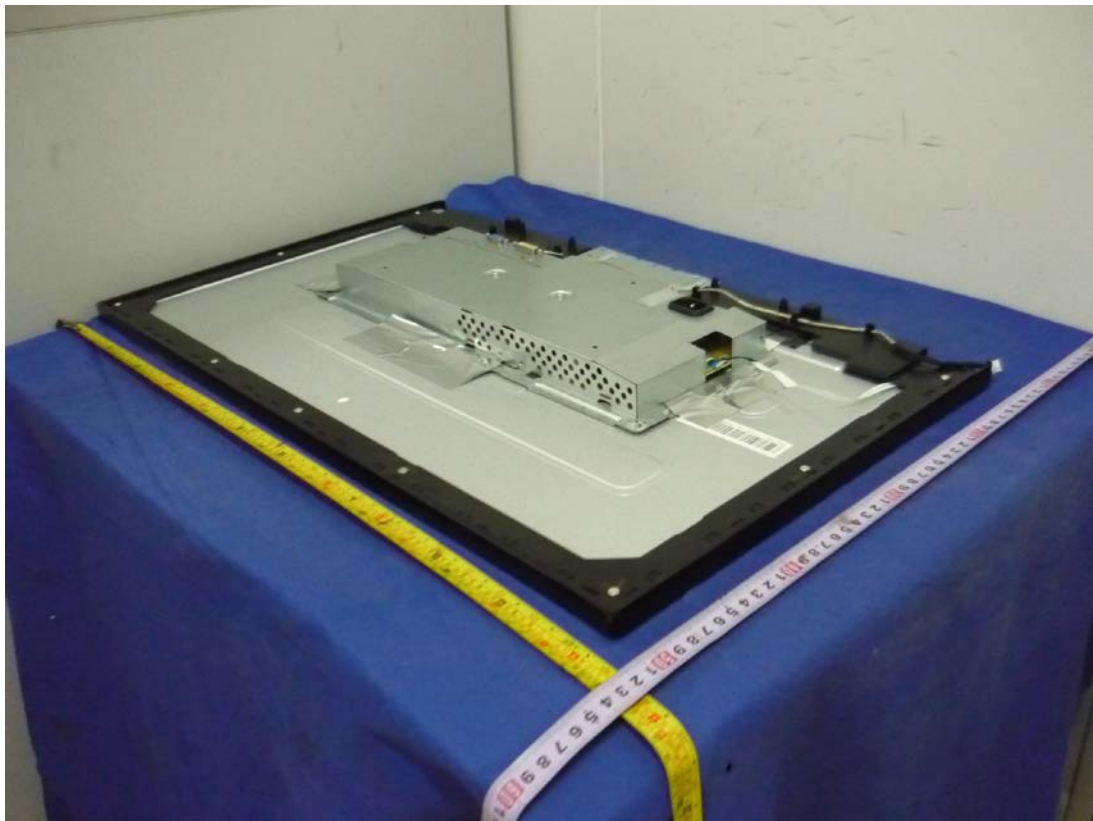
Figure 8. Internal view with main board 715G4502
