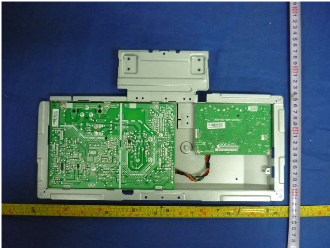
Figure 18. Internal view with main board 715G5811
