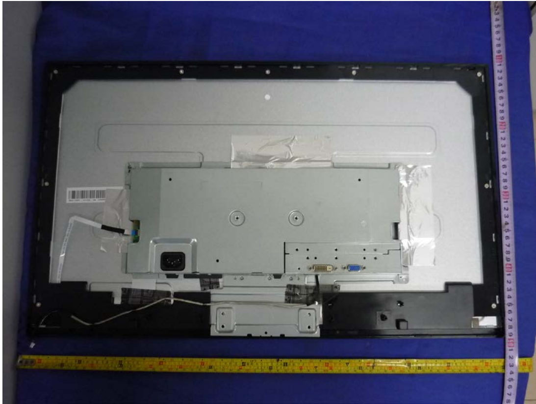
Figure 7. Internal view with main board 715G4502
