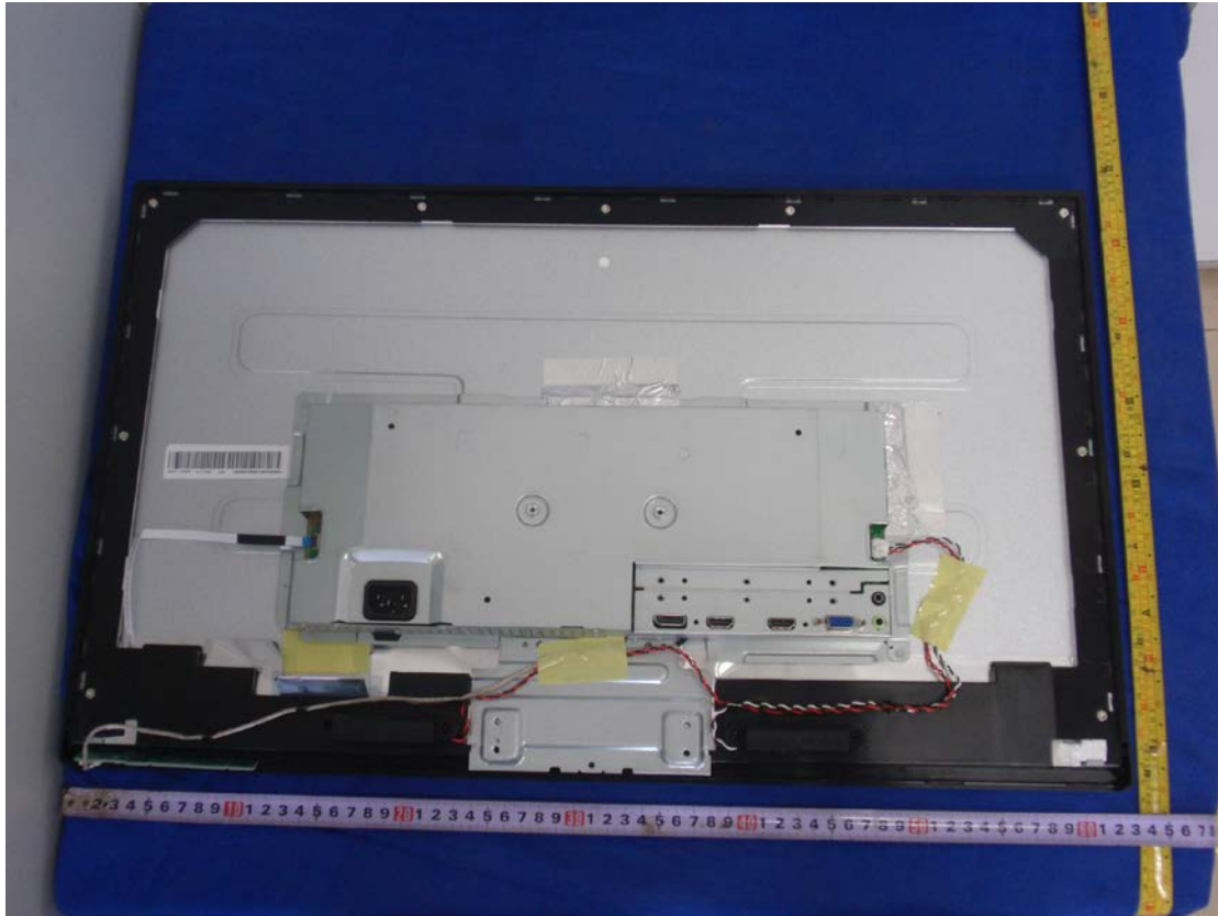
Figure 21. Internal view with main board 715G5812
