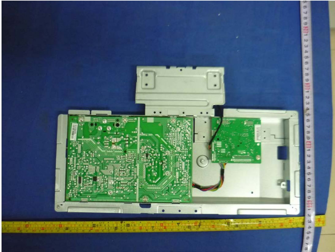
Figure 12. Internal view with main board 715G4502
