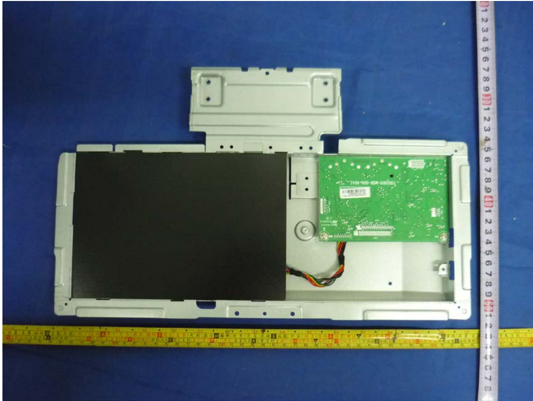
Figure 17. Internal view with main board 715G5811
