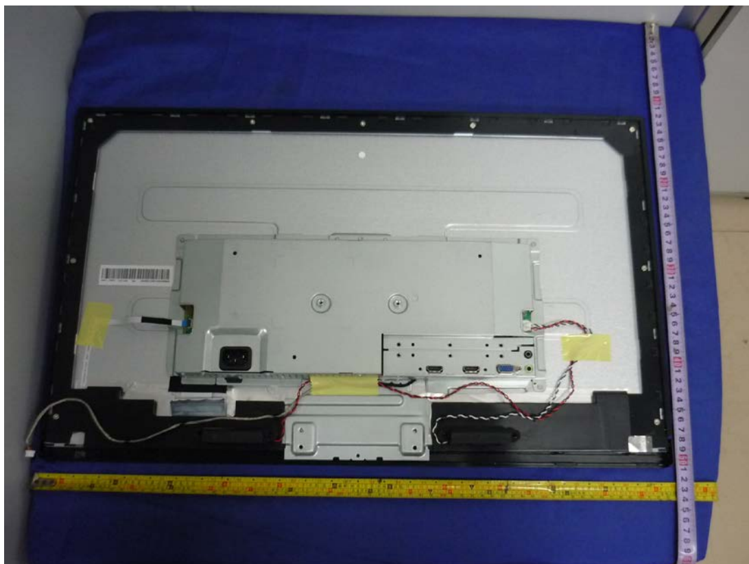
Figure 14. Internal view with main board 715G5811
