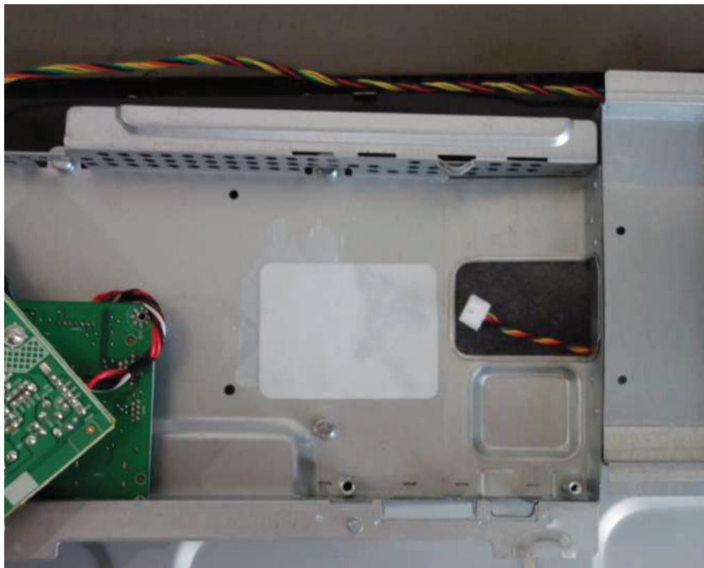
Figure 12. Mylar sheet under power board
