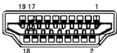
19-Pin Color Display Signal Cable
