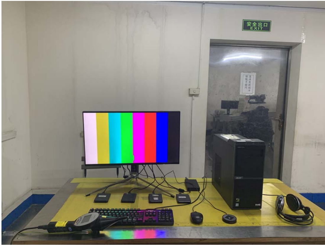
15.5. Photo of RF Strength Susceptibility Test
