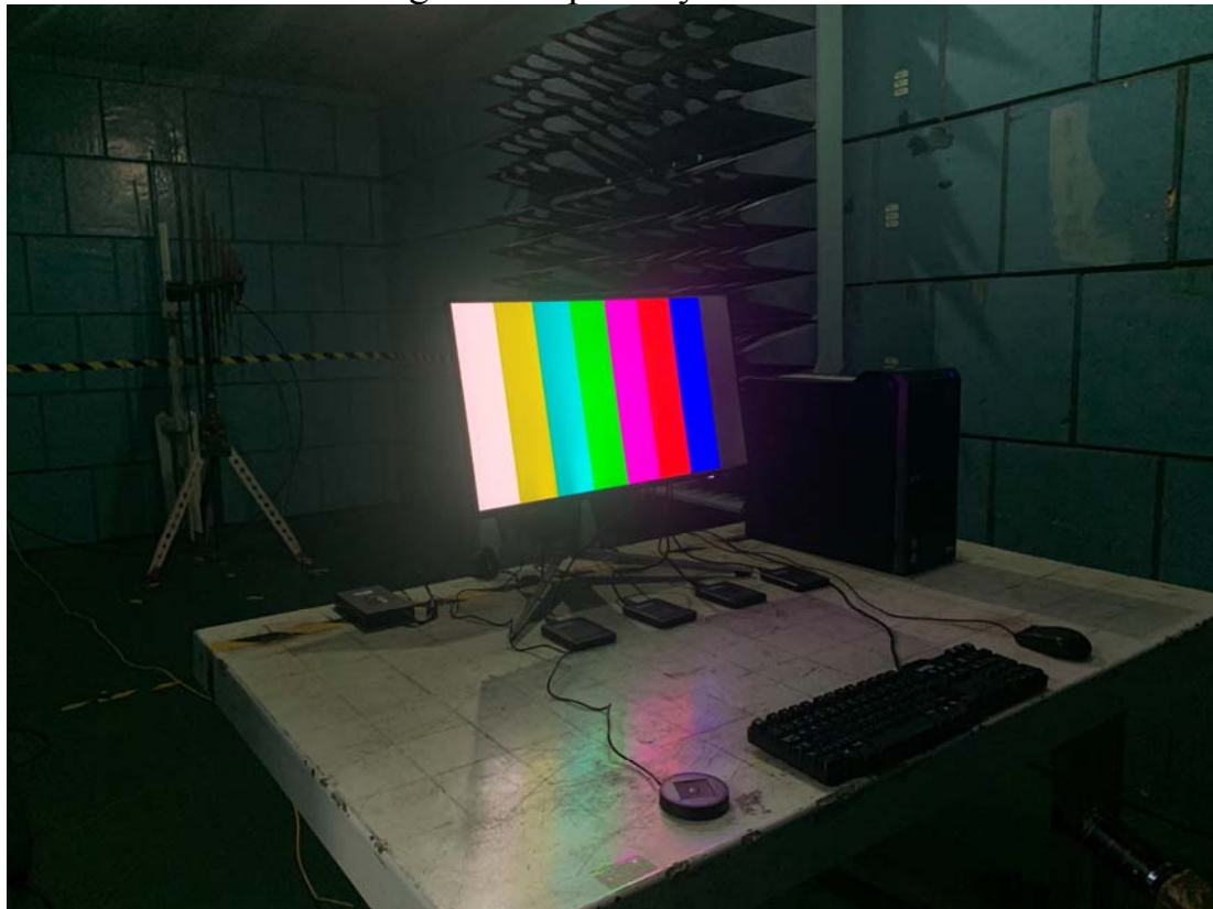
15.5. Photo of RF Strength Susceptibility Test
