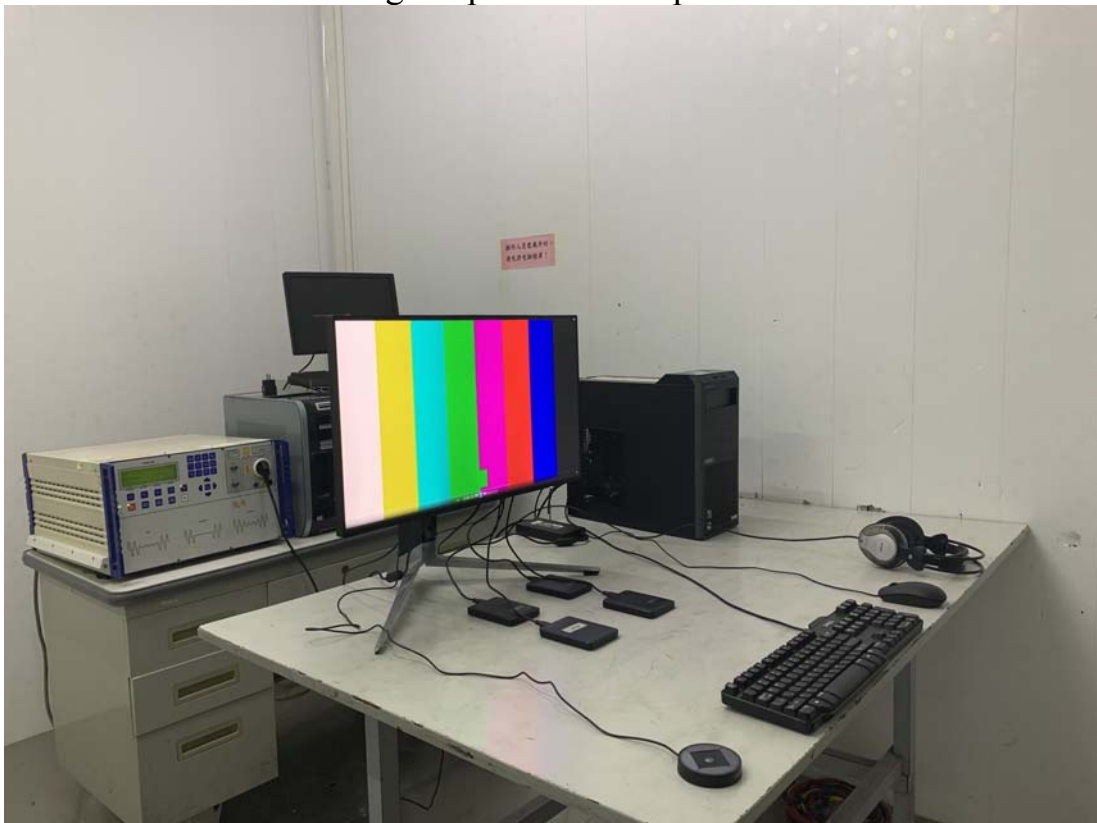
15.10. Photo of Voltage Dips and interruptions test
