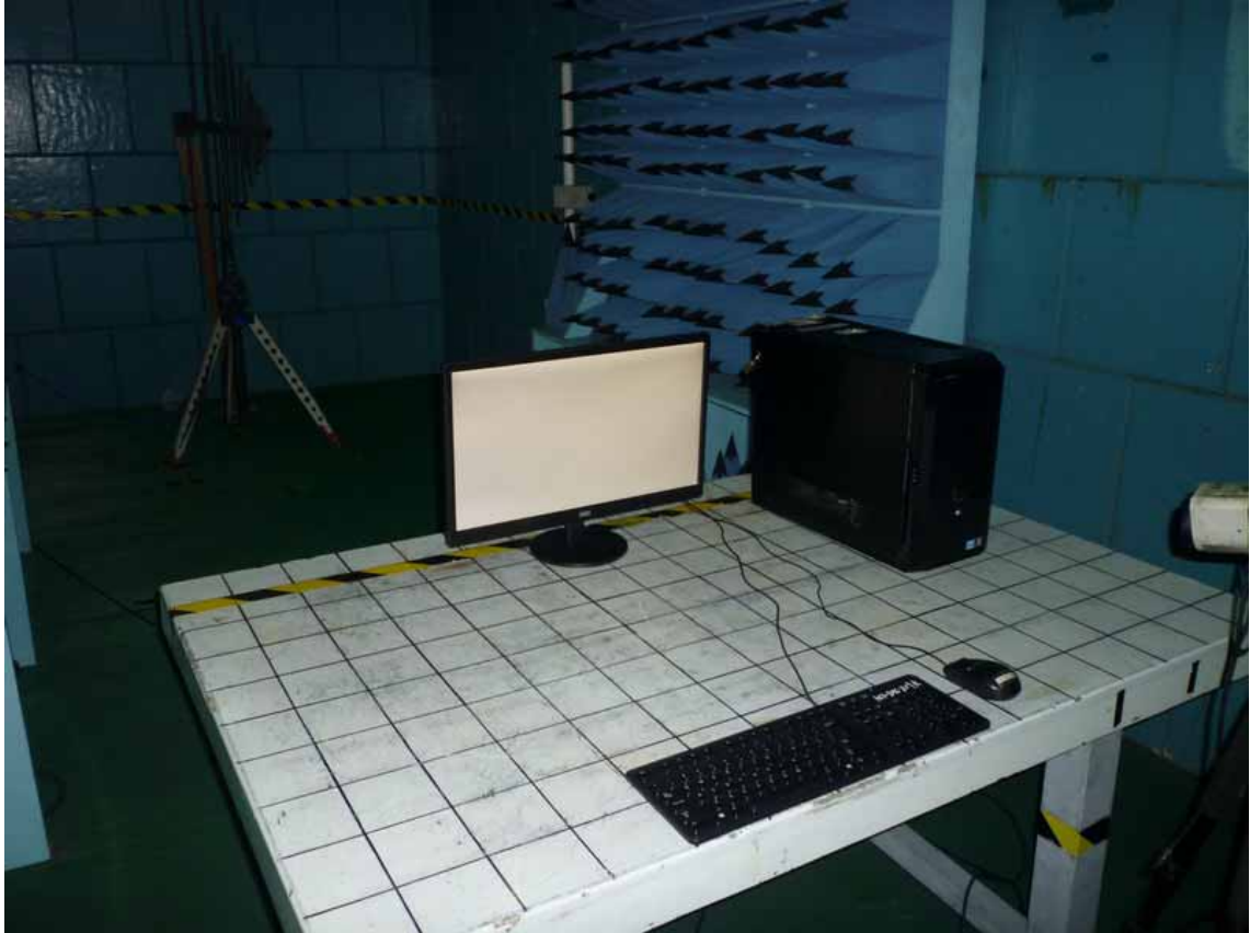
15.5. Photo of RF Strength Susceptibility Test
