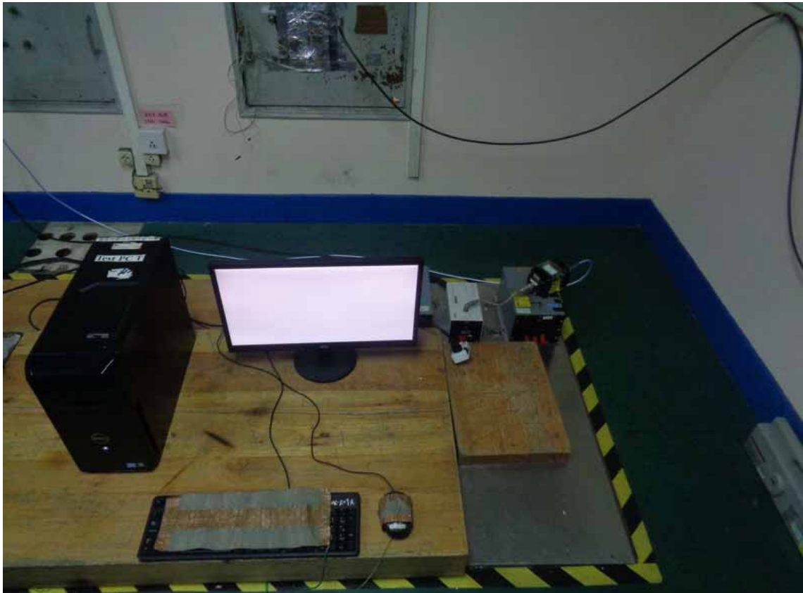
15.8. Photo of Injected Currents Susceptibility Test
