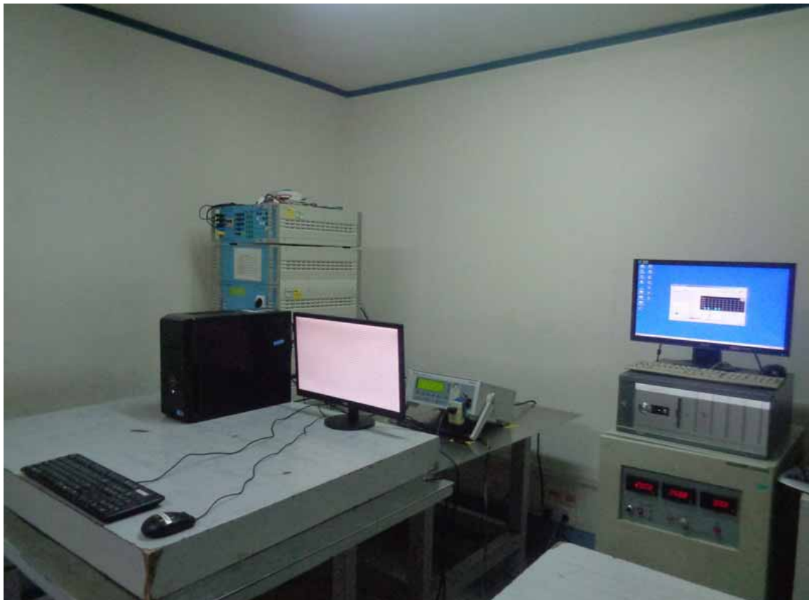
15.6. Photo of Electrical Fast Transient/Burst Immunity Test
