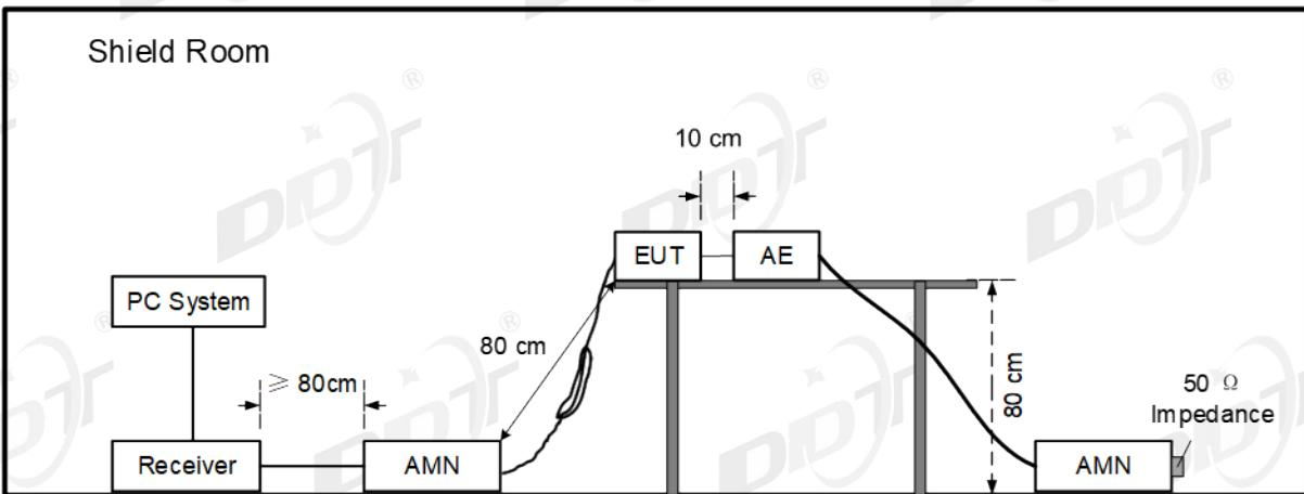
The EUT was placed on a non-metallic table, 80cm above the ground plane. The EUT's power adapter was connected to the power mains through a line impedance stabilization network (AMN), which provided a 50-ohm coupling impedance for the EUT (Please refer to the block diagram of the test setup and photographs). Both sides of power line
