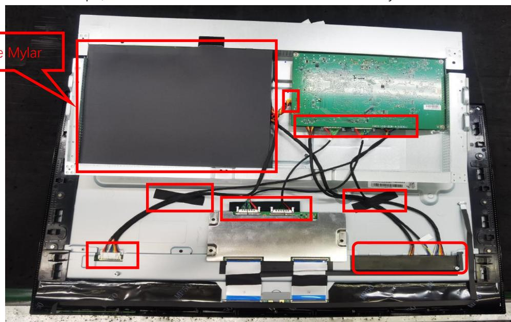
4. Remove the screws to get main board and power board.
