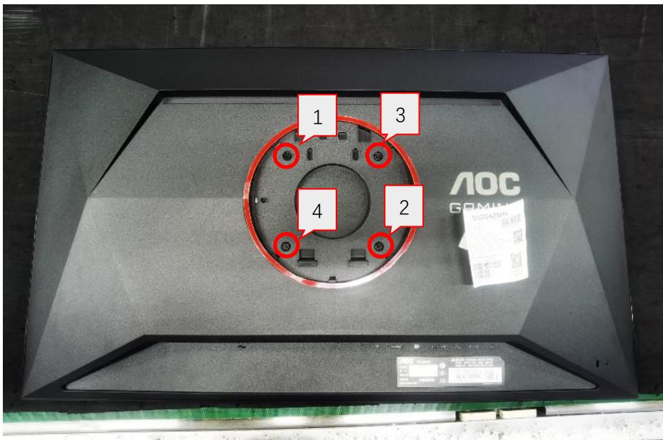
2. Tear off the tape, Disconnect the connection and remove the screws
