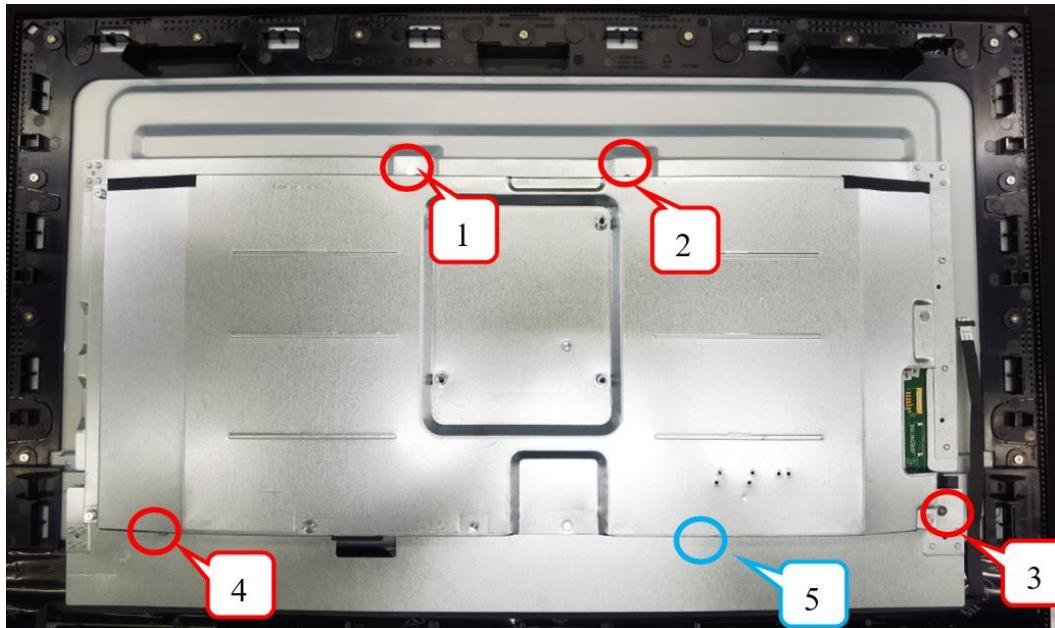
3. Tear off the tape, disconnect the connection and remove the Mylar.
