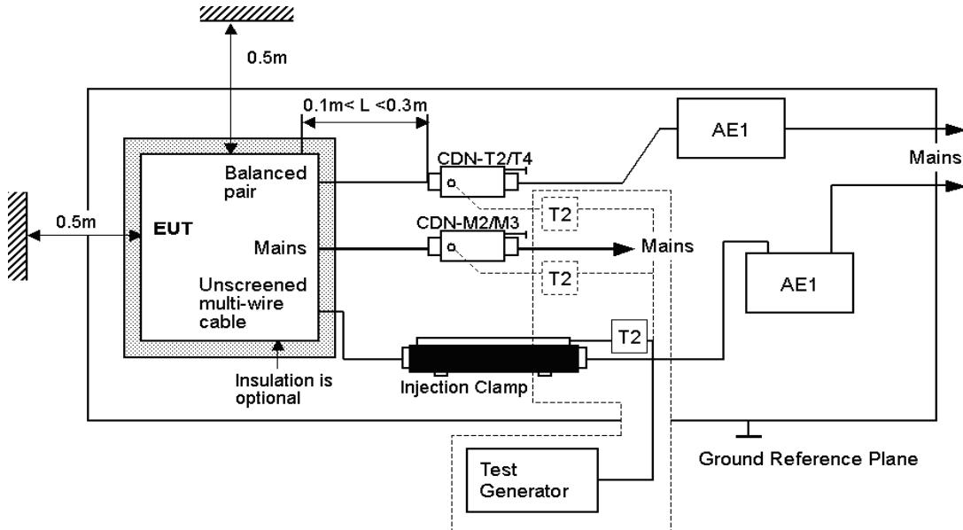
NOTE: The EUT clearance from any metallic obstacles shall be at least 0.5m.
