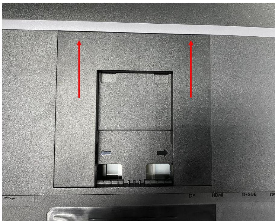
3. Use disassembly tool to open all the latches along the edge of rear cover.
