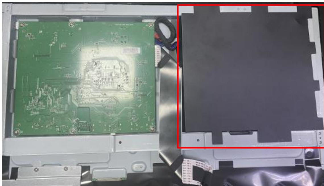
8. Remove screws to get main board and power board.
