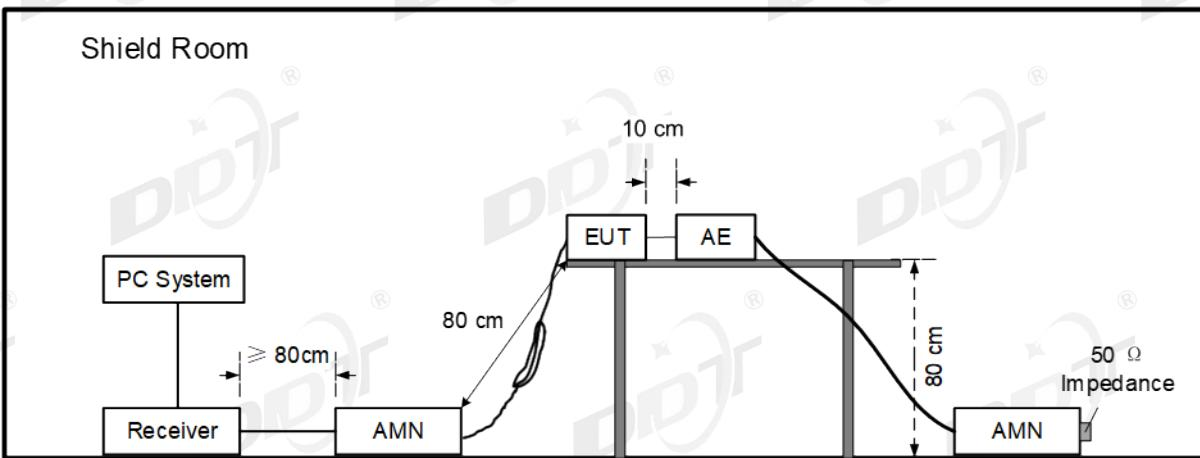
The EUT was placed on a non-metallic table, 80cm above the ground plane.
