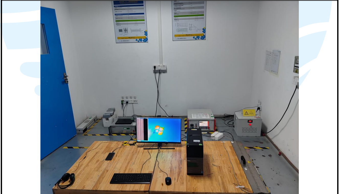
Fast Transients, Common mode (Wired network ports) Test Setup
