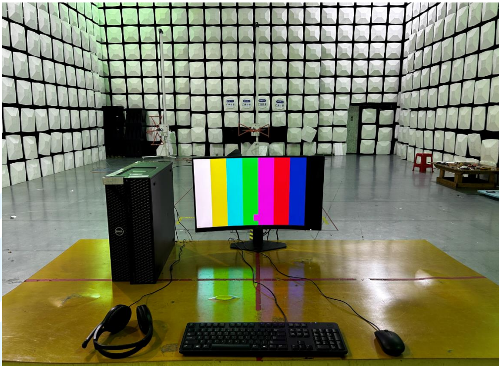
Radiated emission Test Setup (30MHz~1GHz)_ 10 Meter test distance
