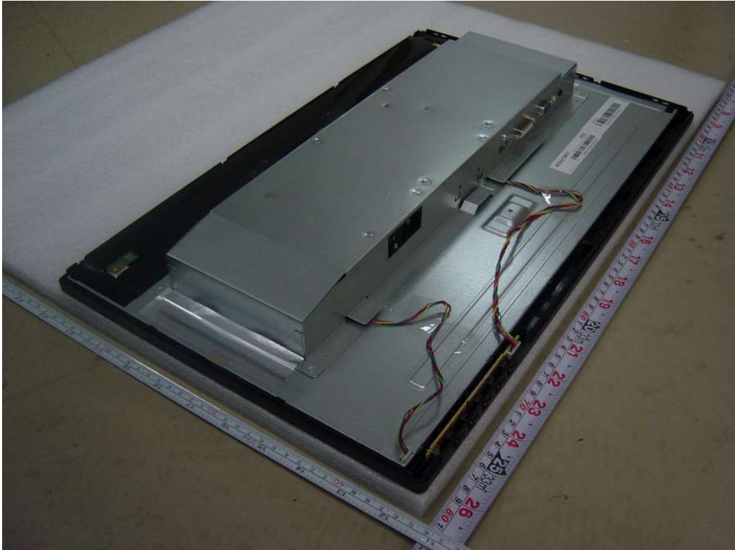
Metal enclosure B with main board B and power supply board (P/N: LE22BW-D-8)
