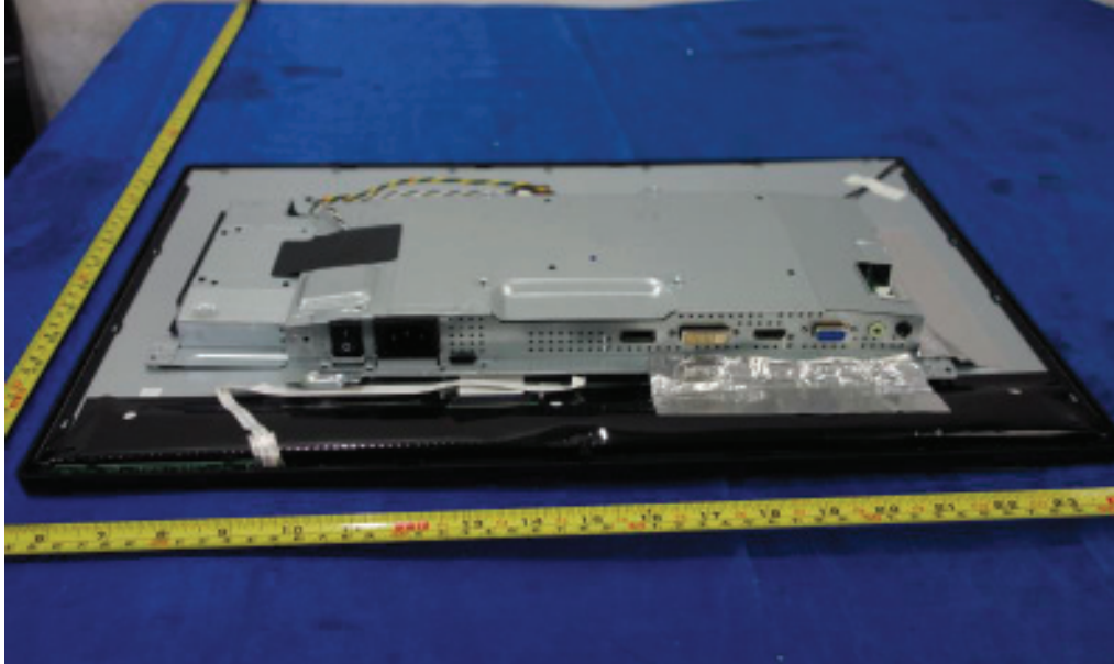
Figure 25. Metal enclosure type D
